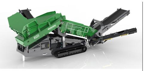
The R155 has proven to be extremely effective across a wide range of applications. With a screening area of 155 ft<sup>2</sup> across the High Energy Screenbox – the largest in its class – the R155 has impressed operators across applications like site reclamation, construction and demolition waste, working with difficult materials such as heavy rock, sticky clay and fines, and boulder clay.
